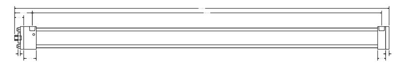
Cylinders Now Model No: CHEARF36CCK54 Logis No: CHEARF36CCK54 Rod End Threas Fonate 7/16 - 20 x 3/4 Bore: 2' Shaft Da: 5/8' MPT Pont Size: 3/8 Mount: RT Stroke: 36 Serbes: 4
