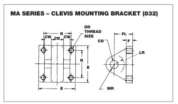
A, MA, HH and MH SERIES: Pins and Retainers supplied with Clevis Mounting Brackets.
