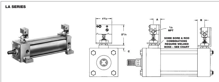
Switches are also available installed in the cap face as shown by **Illustration A**.
