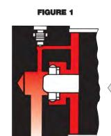
CylindersNow state-of-the-art cushion design features a unique, one-piece, nitrile compound seal that is captured within a precision machined groove. This allows both linear and radial "float" of the cushion seal which virtually eliminates problems associated with misalignment!
